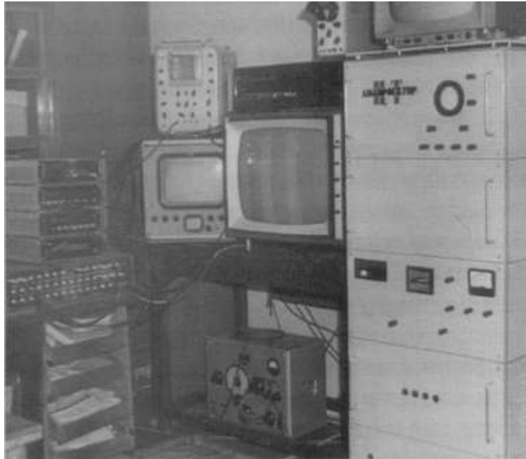
Figure 9. Developed apparatus for experimental broadcasts of color television images (1968 - 1969)
