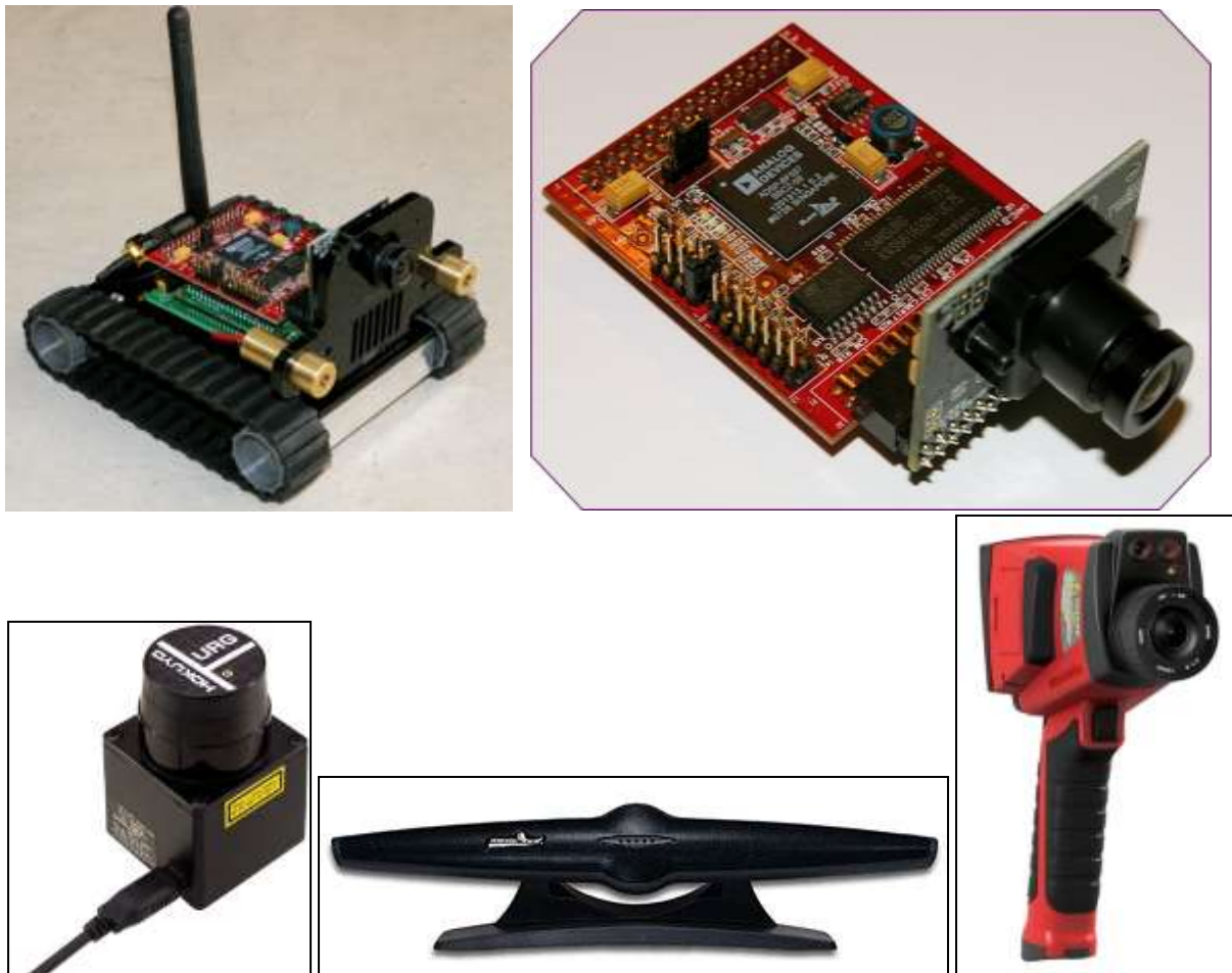
Figure 12. The hardware devices included in the developed audio-visual and thermal imaging systems for motion control of mobile robots
